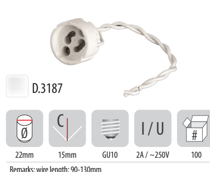
Lamp holder GU10 porcelain LED / halogen
